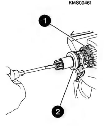
Disassembling overrunning-clutch drive
